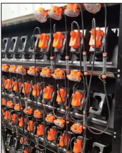
proximity-ready, tracking-enabled and incorporating multiple safety features while having the battery pack worn at the hip. The Falcon continues to provide programmable functionality with two additional buttons to support bidirectional communication and multiple safety features. The Falcon also features the taillight built into the lamp cord to allow others to see the miner ahead.
