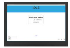
The first time the tag is read, the software will prompt the operator to input the unique serial number engraved on the side of the lamp.
