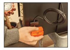
Operator scans the part of the lamp containing the passive RFID tag.
