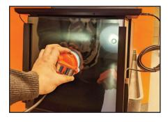
Operator turns the light to its highest setting, placing the lamp on the glass front of the light box and shining the light on the light meter located at the back of the box.
