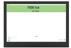
If the light output of the lamp exceeds the easily adjustable pre-set limit set up in the software, the screen will show a green banner indicating a pass and log the lamp's ID, Date, Time and Lux Reading.
